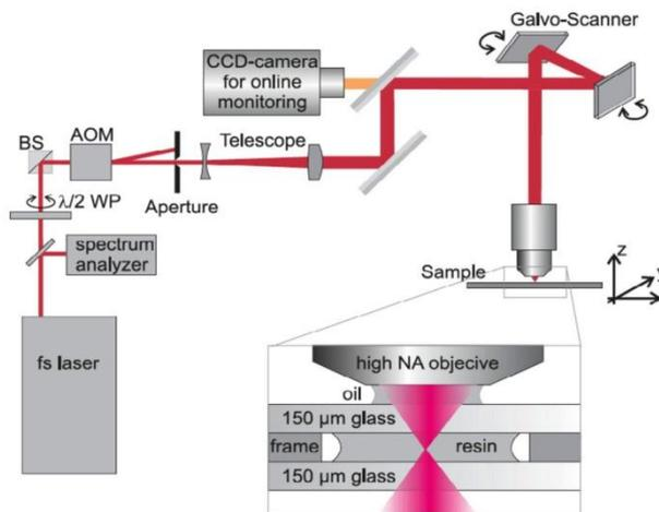
Fig. 1. Schematic of 2PP based 3D structuring
