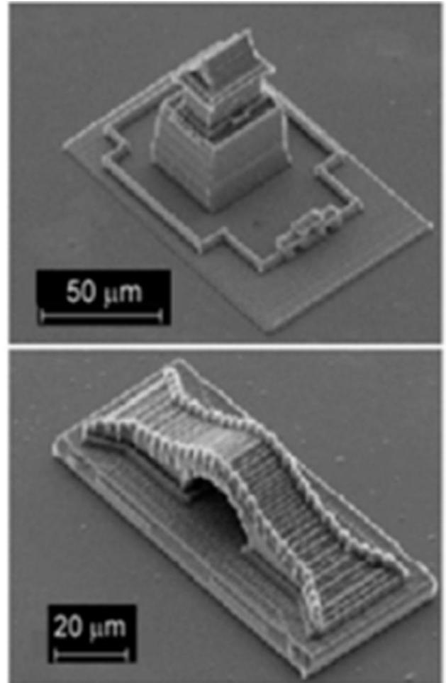
Fig. 3. SEM image of structures build based on 2PP
