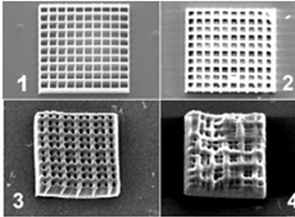
Fig. 3. SEM image of structures built with different laser power. 1 with 9 mW, 2 with 15 mW, 3 with 20 mW and 4 with 27 mW.
