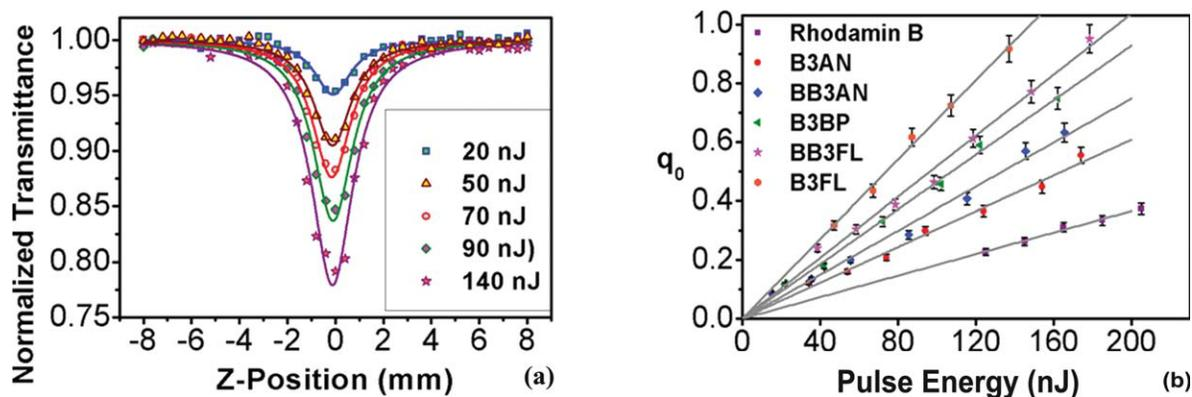
**FIGURE 3** (a) Experimental z-scan data (dots) and fitting curves (full lines) for B 3FL at different pulse energies. (b)  $q_0$  plotted versus intensity for the investigated PIs and an example for standard measurement and fitting data. [Color figure can be viewed in the online issue, which is available at [wileyonlinelibrary.com](http://wileyonlinelibrary.com).]
