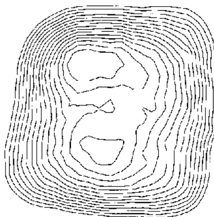
Figure 20 (a) Image of the target spot for a \beta = 4.8 system. (b) Contour plot of the target spot. Contours have equal intervals of 3.2% of the maximum value. (From Ref. 13)
