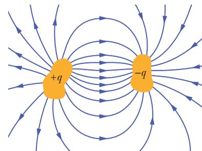
Figure 25-2 Two conductors, isolated electrically from each other and from their surroundings, form a *capacitor*. When the capacitor is charged, the charges on the conductors, or *plates* as they are called, have the same magnitude  $q$  but opposite signs.
