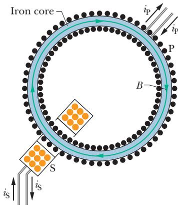
**Figure 32-15** A Rowland ring. A primary coil P has a core made of the ferromagnetic material to be studied (here iron). The core is magnetized by a current  $i_p$  sent through coil P. (The turns of the coil are represented by dots.) The extent to which the core is magnetized determines the total magnetic field  $\vec{B}$  within coil P. Field  $\vec{B}$  can be measured by means of a secondary coil S.
