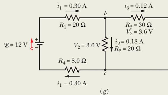
**Figure 27-11** (a) A circuit with an ideal battery. (b) Label the currents. (c) Replacing the parallel resistors with their equivalent. (d)–(g) Working backward to find the currents through the parallel resistors.
