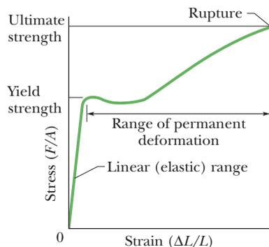
**Figure 12-13** A stress–strain curve for a steel test specimen such as that of Fig. 12-12. The specimen deforms permanently when the stress is equal to the *yield strength* of the specimen's material. It ruptures when the stress is equal to the *ultimate strength* of the material.
