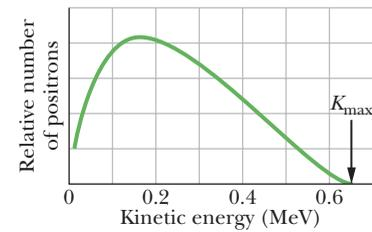
**Figure 42-11** The distribution of the kinetic energies of positrons emitted in the beta decay of  $^{64}\text{Cu}$ . The maximum kinetic energy of the distribution ( $K_{\max}$ ) is 0.653 MeV. In all  $^{64}\text{Cu}$  decay events, this energy is shared between the positron and the neutrino, in varying proportions. The *most probable* energy for an emitted positron is about 0.15 MeV.
