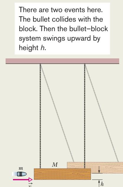
**Figure 9-17** A ballistic pendulum, used to measure the speeds of bullets.
