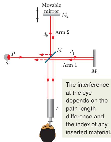
**Figure 35-21** Michelson's interferometer, showing the path of light originating at point  $P$  of an extended source  $S$ . Mirror  $M$  splits the light into two beams, which reflect from mirrors  $M_1$  and  $M_2$  back to  $M$  and then to telescope  $T$ . In the telescope an observer sees a pattern of interference fringes.
