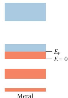
**Figure 41-5** The band-gap pattern for a metal. The highest filled level, called the Fermi level, lies near the middle of a band. Since vacant levels are available within that band, electrons in the band can easily change levels, and conduction can take place.
