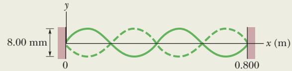
Figure 16-23 Resonant oscillation of a string under tension.
