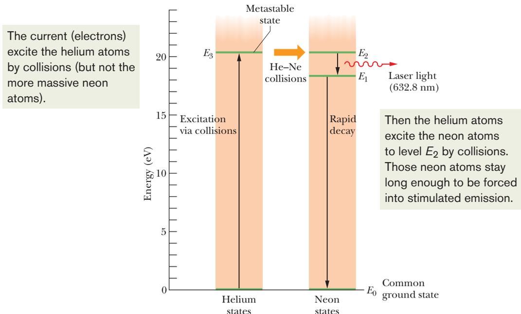
**Figure 40-21** Five essential energy levels for helium and neon atoms in a helium–neon gas laser. Laser action occurs between levels  $E_2$  and  $E_1$  of neon when more atoms are at the  $E_2$  level than at the  $E_1$  level.
