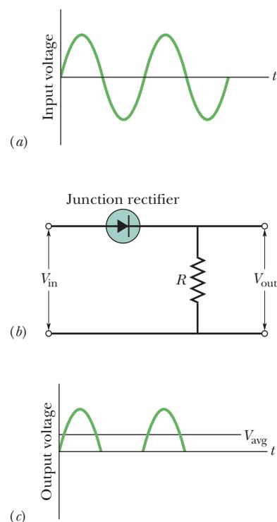
**Figure 41-14** A *p-n* junction connected as a junction rectifier. The action of the circuit in (b) is to pass the positive half of the input wave form in (a) but to suppress the negative half. The average potential of the input wave form is zero; that of the output wave form in (c) has a positive value  $V_{\text{avg}}$ .
