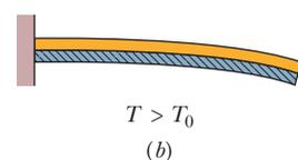
**Figure 18-10** (a) A bimetal strip, consisting of a strip of brass and a strip of steel welded together, at temperature  $T_0$ . (b) The strip bends as shown at temperatures above this reference temperature. Below the reference temperature the strip bends the other way. Many thermostats operate on this principle, making and breaking an electrical contact as the temperature rises and falls.
