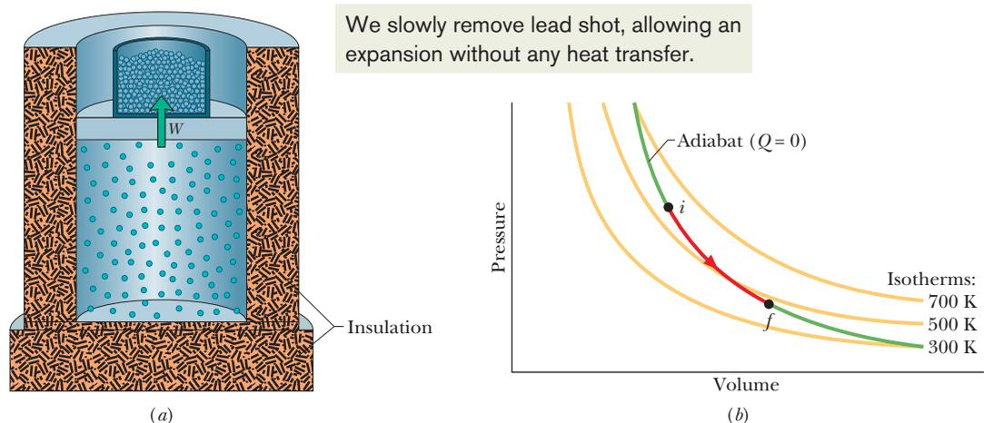
**Figure 19-15** (a) The volume of an ideal gas is increased by removing mass from the piston. The process is adiabatic ( $Q = 0$ ). (b) The process proceeds from  $i$  to  $f$  along an adiabat on a  $p$ - $V$  diagram.
