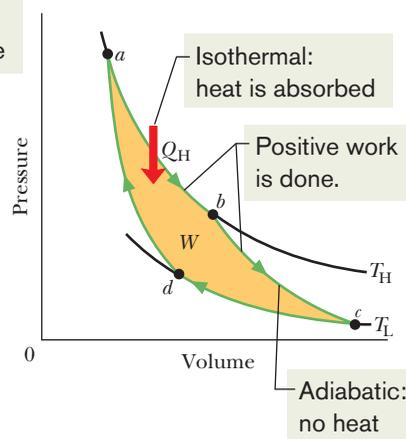
**Figure 20-9** A pressure–volume plot of the cycle followed by the working substance of the Carnot engine in Fig. 20-8. The cycle consists of two isothermal ( $ab$  and  $cd$ ) and two adiabatic processes ( $bc$  and  $da$ ). The shaded area enclosed by the cycle is equal to the work  $W$  per cycle done by the Carnot engine.
