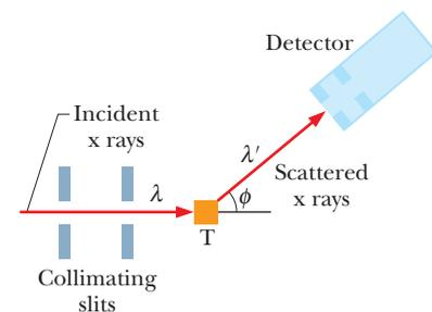
**Figure 38-3** Compton's apparatus. A beam of x rays of wavelength  $\lambda = 71.1$  pm is directed onto a carbon target T. The x rays scattered from the target are observed at various angles  $\phi$  to the direction of the incident beam. The detector measures both the intensity of the scattered x rays and their wavelength.
