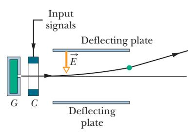
**Figure 22-17** Ink-jet printer. Drops shot from generator  $G$  receive a charge in charging unit  $C$ . An input signal from a computer controls the charge and thus the effect of field  $\vec{E}$  on where the drop lands on the paper.
