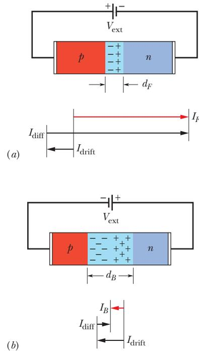
**Figure 41-15** (a) The forward-bias connection of a  $p$ - $n$  junction, showing the narrowed depletion zone and the large forward current  $I_F$ . (b) The back-bias connection, showing the widened depletion zone and the small back current  $I_B$ .
