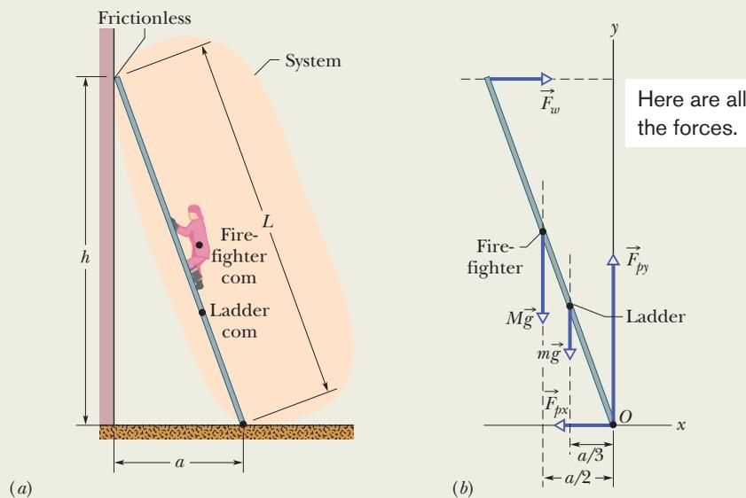
**Figure 12-7** (a) A firefighter climbs halfway up a ladder that is leaning against a frictionless wall. The pavement beneath the ladder is not frictionless. (b) A free-body diagram, showing the forces that act on the firefighter + ladder system. The origin  $O$  of a coordinate system is placed at the point of application of the unknown force  $\vec{F}_p$  (whose vector components  $\vec{F}_{px}$  and  $\vec{F}_{py}$  are shown). (Figure 12-7 continues on following page.)
