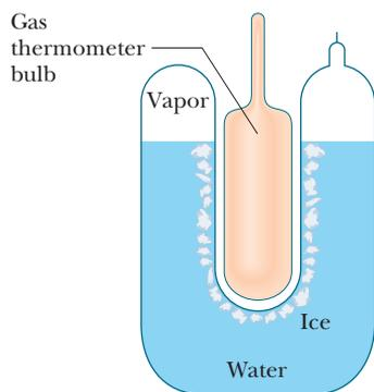
**Figure 18-4** A triple-point cell, in which solid ice, liquid water, and water vapor coexist in thermal equilibrium. By international agreement, the temperature of this mixture has been defined to be 273.16 K. The bulb of a constant-volume gas thermometer is shown inserted into the well of the cell.
