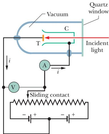
**Figure 38-1** An apparatus used to study the photoelectric effect. The incident light shines on target T, ejecting electrons, which are collected by collector cup C. The electrons move in the circuit in a direction opposite the conventional current arrows. The batteries and the variable resistor are used to produce and adjust the electric potential difference between T and C.
