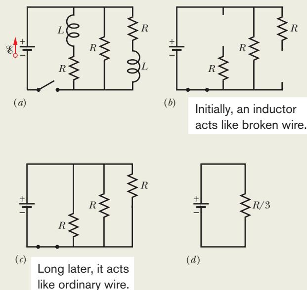
**Figure 30-18** (a) A multiloop *RL* circuit with an open switch. (b) The equivalent circuit just after the switch has been closed. (c) The equivalent circuit a long time later. (d) The single-loop circuit that is equivalent to circuit (c).
