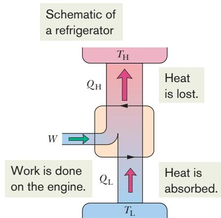
**Figure 20-14** The elements of a refrigerator. The two black arrowheads on the central loop suggest the working substance operating in a cycle, as if on a  $p$ - $V$  plot. Energy is transferred as heat  $Q_L$  to the working substance from the low-temperature reservoir. Energy is transferred as heat  $Q_H$  to the high-temperature reservoir from the working substance. Work  $W$  is done on the refrigerator (on the working substance) by something in the environment.
