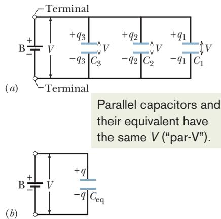
**Figure 25-8** (a) Three capacitors connected in parallel to battery B. The battery maintains potential difference  $V$  across its terminals and thus across *each* capacitor. (b) The equivalent capacitor, with capacitance  $C_{eq}$ , replaces the parallel combination.
