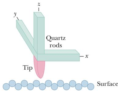
**Figure 38-19** The essence of a scanning tunneling microscope (STM). Three quartz rods are used to scan a sharply pointed conducting tip across the surface of interest and to maintain a constant separation between tip and surface. The tip thus moves up and down to match the contours of the surface, and a record of its movement provides information for a computer to create an image of the surface.
