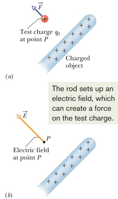
**Figure 22-2** (a) A positive test charge  $q_0$  placed at point  $P$  near a charged object. An electrostatic force  $\vec{F}$  acts on the test charge. (b) The electric field  $\vec{E}$  at point  $P$  produced by the charged object.
