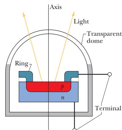
**Figure 41-17** Cross section of an LED (the device has rotational symmetry about the central axis). The  $p$ -type material, which is thin enough to transmit light, is in the form of a circular disk. A connection is made to the  $p$ -type material through a circular metal ring that touches the disk at its periphery. The depletion zone between the  $n$ -type material and the  $p$ -type material is not shown.
