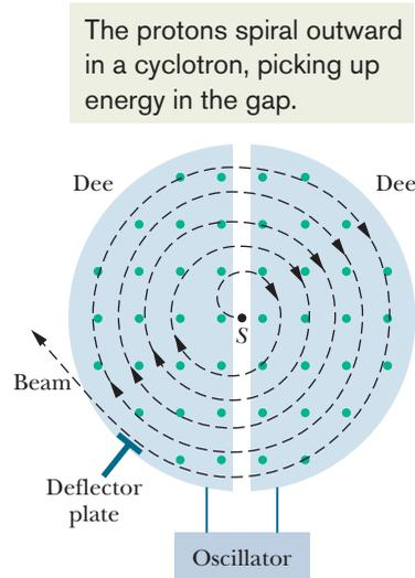
**Figure 28-13** The elements of a cyclotron, showing the particle source  $S$  and the dees. A uniform magnetic field is directed up from the plane of the page. Circulating protons spiral outward within the hollow dees, gaining energy every time they cross the gap between the dees.
