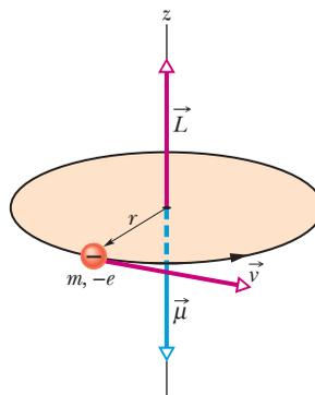
**Figure 40-3** A classical model showing a particle of mass  $m$  and charge  $-e$  moving with speed  $v$  in a circle of radius  $r$ . The moving particle has an angular momentum  $\vec{L}$  given by  $\vec{r} \times \vec{p}$ , where  $\vec{p}$  is its linear momentum  $m\vec{v}$ . The particle's motion is equivalent to a current loop that has an associated magnetic moment  $\vec{\mu}$  that is directed opposite  $\vec{L}$ .
