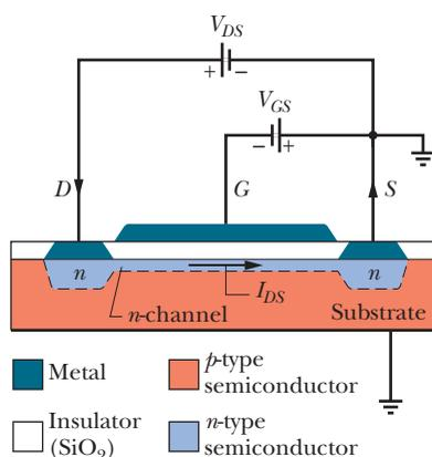
**Figure 41-20** A particular type of field-effect transistor known as a MOSFET. The magnitude of the drain-to-source conventional current  $I_{DS}$  through the  $n$  channel is controlled by the potential difference  $V_{GS}$  applied between the source  $S$  and the gate  $G$ . A depletion zone that exists between the  $n$ -type material and the  $p$ -type substrate is not shown.
