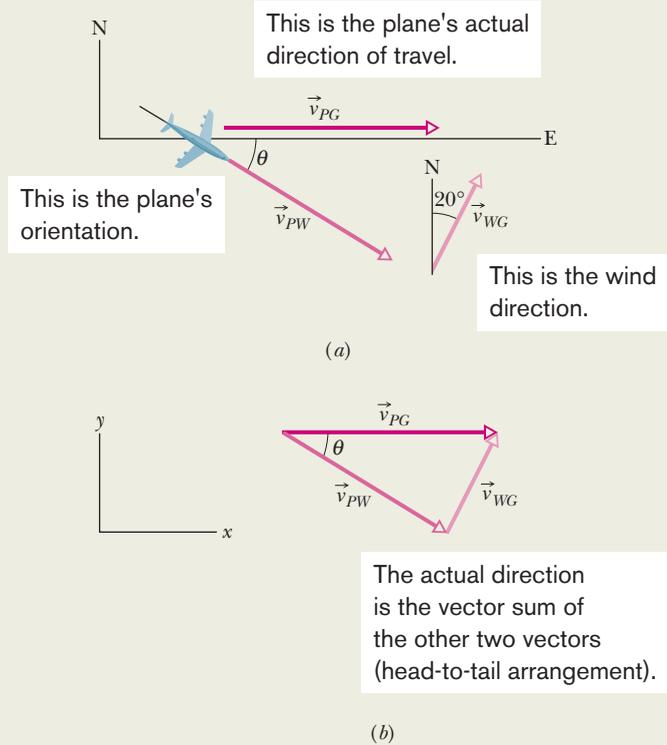
Figure 4-20 A plane flying in a wind.
