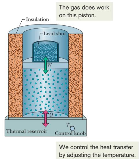
**Figure 18-13** A gas is confined to a cylinder with a movable piston. Heat  $Q$  can be added to or withdrawn from the gas by regulating the temperature  $T$  of the adjustable thermal reservoir. Work  $W$  can be done by the gas by raising or lowering the piston.
