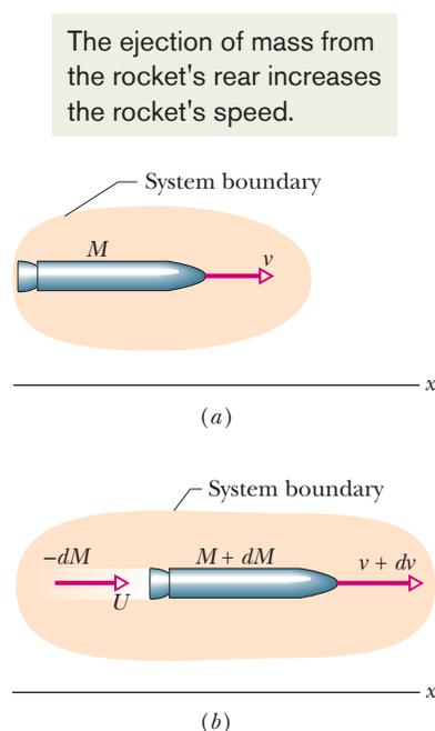
**Figure 9-22** (a) An accelerating rocket of mass  $M$  at time  $t$ , as seen from an inertial reference frame. (b) The same but at time  $t + dt$ . The exhaust products released during interval  $dt$  are shown.
