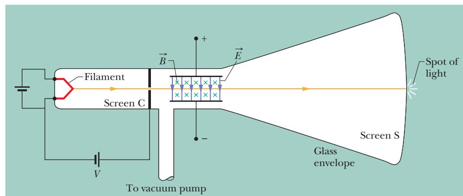
**Figure 28-7** A modern version of J. J. Thomson's apparatus for measuring the ratio of mass to charge for the electron. An electric field  $\vec{E}$  is established by connecting a battery across the deflecting-plate terminals. The magnetic field  $\vec{B}$  is set up by means of a current in a system of coils (not shown). The magnetic field shown is into the plane of the figure, as represented by the array of **X**s (which resemble the feathered ends of arrows).
