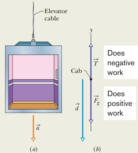
**Figure 7-9** An elevator cab, descending with speed  $v_i$ , suddenly begins to accelerate downward. (a) It moves through a displacement  $\vec{d}$  with constant acceleration  $\vec{a} = \vec{g}/5$ . (b) A free-body diagram for the cab, displacement included.
