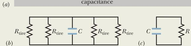
**Figure 27-17** (a) A charged car and the pavement acts like a capacitor that can discharge through the tires. (b) The effective circuit of the car–pavement capacitor, with four tire resistances  $R_{\text{tire}}$  connected in parallel. (c) The equivalent resistance  $R$  of the tires. (d) The electric potential energy  $U$  in the car–pavement capacitor decreases during discharge.
