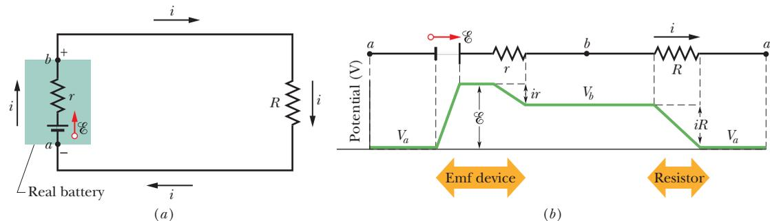
**Figure 27-4** (a) A single-loop circuit containing a real battery having internal resistance  $r$  and emf  $\mathcal{E}$ . (b) The same circuit, now spread out in a line. The potentials encountered in traversing the circuit clockwise from  $a$  are also shown. The potential  $V_a$  is arbitrarily assigned a value of zero, and other potentials in the circuit are graphed relative to  $V_a$ .
