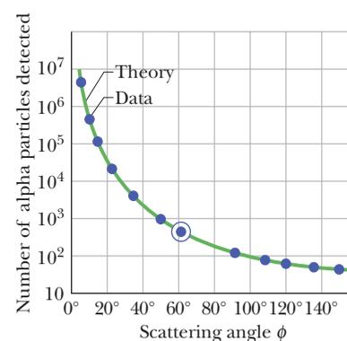
**Figure 42-2** The dots are alpha-particle scattering data for a gold foil, obtained by Geiger and Marsden using the apparatus of Fig. 42-1. The solid curve is the theoretical prediction, based on the assumption that the atom has a small, massive, positively charged nucleus. The data have been adjusted to fit the theoretical curve at the experimental point that is enclosed in a circle.
