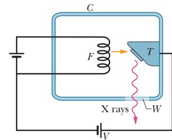
**Figure 36-27** X rays are generated when electrons leaving heated filament  $F$  are accelerated through a potential difference  $V$  and strike a metal target  $T$ . The “window”  $W$  in the evacuated chamber  $C$  is transparent to x rays.
