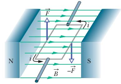
**Figure 28-18** The elements of an electric motor. A rectangular loop of wire, carrying a current and free to rotate about a fixed axis, is placed in a magnetic field. Magnetic forces on the wire produce a torque that rotates it. A commutator (not shown) reverses the direction of the current every half-revolution so that the torque always acts in the same direction.
