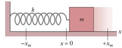
**Figure 15-7** A linear simple harmonic oscillator. The surface is frictionless. Like the particle of Fig. 15-2, the block moves in simple harmonic motion once it has been either pulled or pushed away from the  $x = 0$  position and released. Its displacement is then given by Eq. 15-3.
