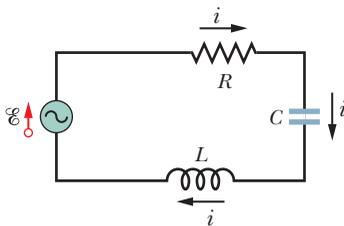
**Figure 31-7** A single-loop circuit containing a resistor, a capacitor, and an inductor. A generator, represented by a sine wave in a circle, produces an alternating emf that establishes an alternating current; the directions of the emf and current are indicated here at only one instant.
