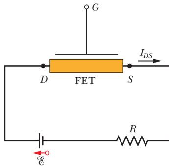
**Figure 41-19** A circuit containing a generalized field-effect transistor through which electrons flow from the source terminal  $S$  to the drain terminal  $D$ . (The conventional current  $I_{DS}$  is in the opposite direction.) The magnitude of  $I_{DS}$  is controlled by the electric field set up within the FET by a potential applied to  $G$ , the gate terminal.
