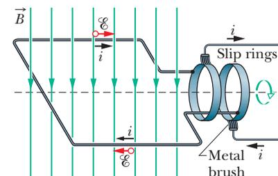
**Figure 31-6** The basic mechanism of an alternating-current generator is a conducting loop rotated in an external magnetic field. In practice, the alternating emf induced in a coil of many turns of wire is made accessible by means of slip rings attached to the rotating loop. Each ring is connected to one end of the loop wire and is electrically connected to the rest of the generator circuit by a conducting brush against which the ring slips as the loop (and it) rotates.
