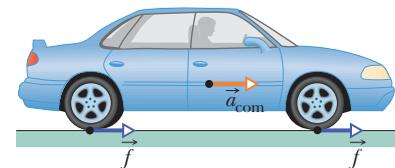
**Figure 8-16** A vehicle accelerates to the right using four-wheel drive. The road exerts four frictional forces (two of them shown) on the bottom surfaces of the tires. Taken together, these four forces make up the net external force  $\vec{F}$  acting on the car.
