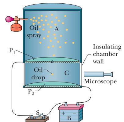
**Figure 22-16** The Millikan oil-drop apparatus for measuring the elementary charge  $e$ . When a charged oil drop drifted into chamber C through the hole in plate  $P_1$ , its motion could be controlled by closing and opening switch  $S$  and thereby setting up or eliminating an electric field in chamber C. The microscope was used to view the drop, to permit timing of its motion.
