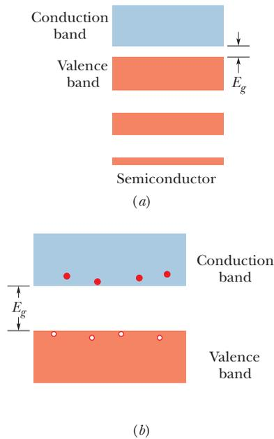
**Figure 41-9** (a) The band-gap pattern for a semiconductor. It resembles that of an insulator (see Fig. 41-4) except that here the energy gap  $E_g$  is much smaller; thus electrons, because of their thermal agitation, have some reasonable probability of being able to jump the gap. (b) Thermal agitation has caused a few electrons to jump the gap from the valence band to the conduction band, leaving an equal number of holes in the valence band.
