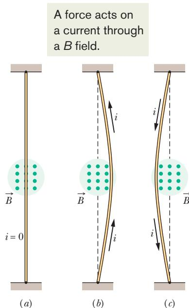
**Figure 28-14** A flexible wire passes between the pole faces of a magnet (only the farther pole face is shown). (a) Without current in the wire, the wire is straight. (b) With upward current, the wire is deflected rightward. (c) With downward current, the deflection is leftward. The connections for getting the current into the wire at one end and out of it at the other end are not shown.
