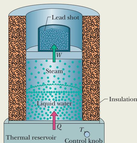
**Figure 18-17** Water boiling at constant pressure. Energy is transferred from the thermal reservoir as heat until the liquid water has changed completely into steam. Work is done by the expanding gas as it lifts the loaded piston.
