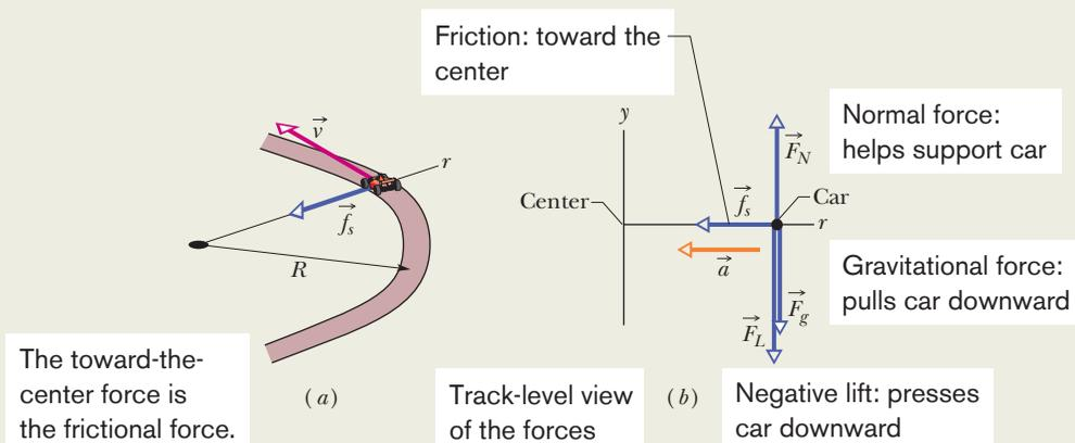
**Figure 6-10** (a) A race car moves around a flat curved track at constant speed  $v$ . The frictional force  $\vec{f}_s$  provides the necessary centripetal force along a radial axis  $r$ . (b) A free-body diagram (not to scale) for the car, in the vertical plane containing  $r$ .
