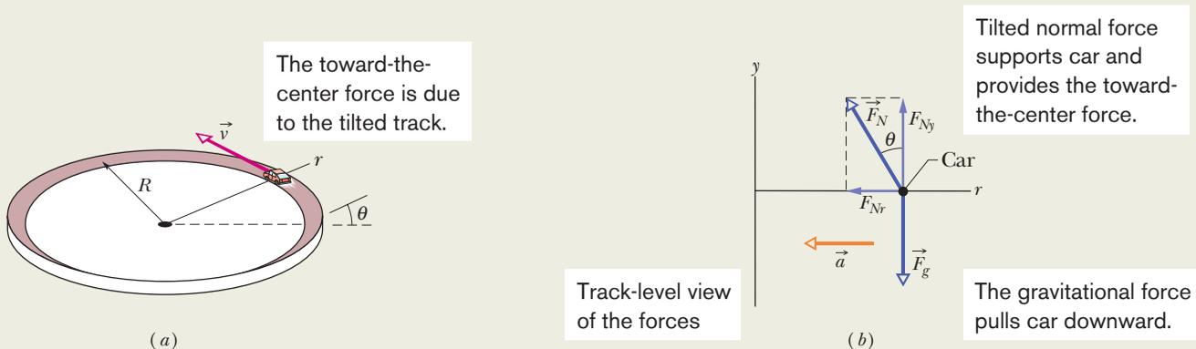
**Figure 6-11** (a) A car moves around a curved banked road at constant speed  $v$ . The bank angle is exaggerated for clarity. (b) A free-body diagram for the car, assuming that friction between tires and road is zero and that the car lacks negative lift. The radially inward component  $F_{Nr}$  of the normal force (along radial axis  $r$ ) provides the necessary centripetal force and radial acceleration.
