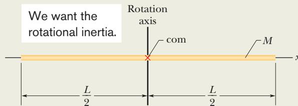
**Figure 10-14** A uniform rod of length  $L$  and mass  $M$ . An element of mass  $dm$  and length  $dx$  is represented.
