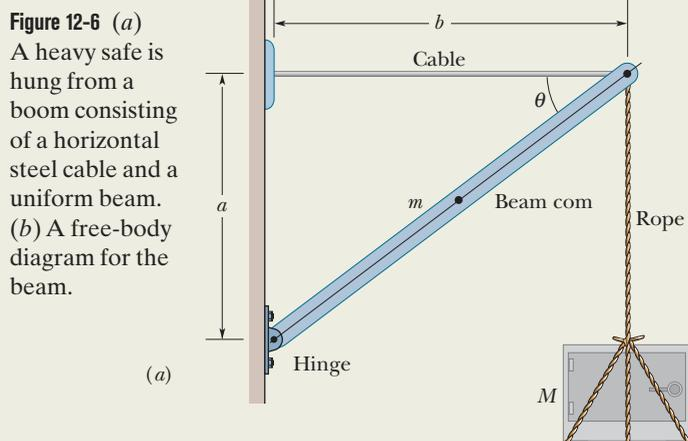
**Figure 12-6** (a) A heavy safe is hung from a boom consisting of a horizontal steel cable and a uniform beam. (b) A free-body diagram for the beam.
