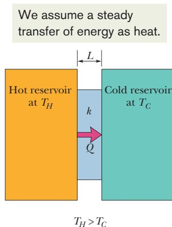
**Figure 18-18** Thermal conduction. Energy is transferred as heat from a reservoir at temperature  $T_H$  to a cooler reservoir at temperature  $T_C$  through a conducting slab of thickness  $L$  and thermal conductivity  $k$ .
