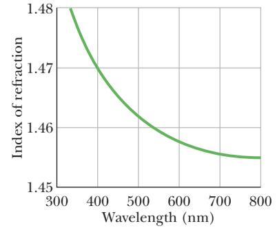
**Figure 33-18** The index of refraction as a function of wavelength for fused quartz. The graph indicates that a beam of short-wavelength light, for which the index of refraction is higher, is bent more upon entering or leaving quartz than a beam of long-wavelength light.
